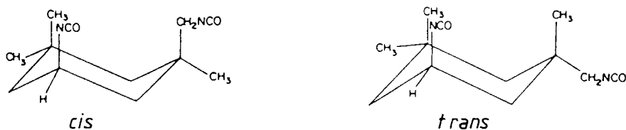
Fig. 2. cis and trans isomers of isophorone diisocyanate.
